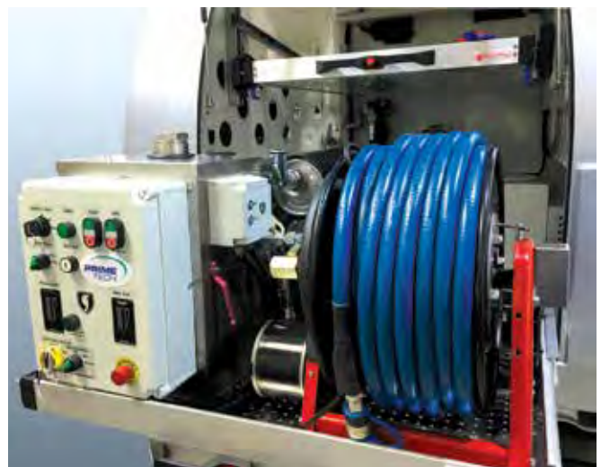
The Primetech MultiPod vehicle is equipped with the MultiPod® COBRA fire fighting system on an up to 300 bar system, delivering a very fine spray into fire spaces, allowing for a safe and highly effective external attack on a building fire
